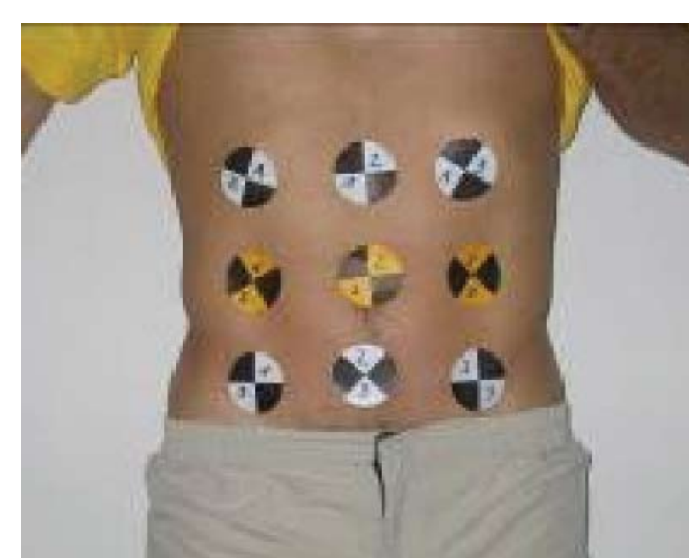
Impactor test on a PMHS lower leg (left) and impact location on a volunteer's abdomen (right)
