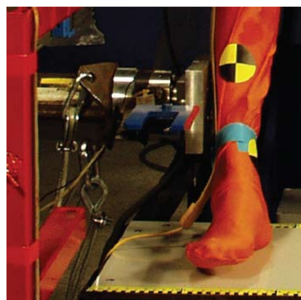
Impactor test on a PMHS lower leg (left) and impact location on a volunteer's abdomen (right)
