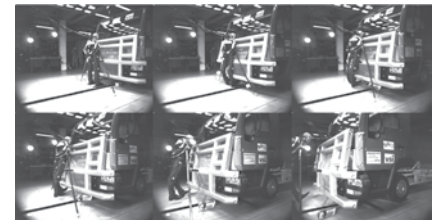
Impact of pedestrian dummy vs. safety bar (30 kph)
