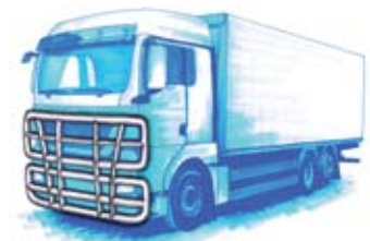
After-market safety bar on a conventional truck (safety & styling)
