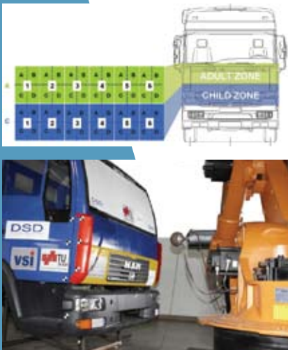
impact zones for structural testing
