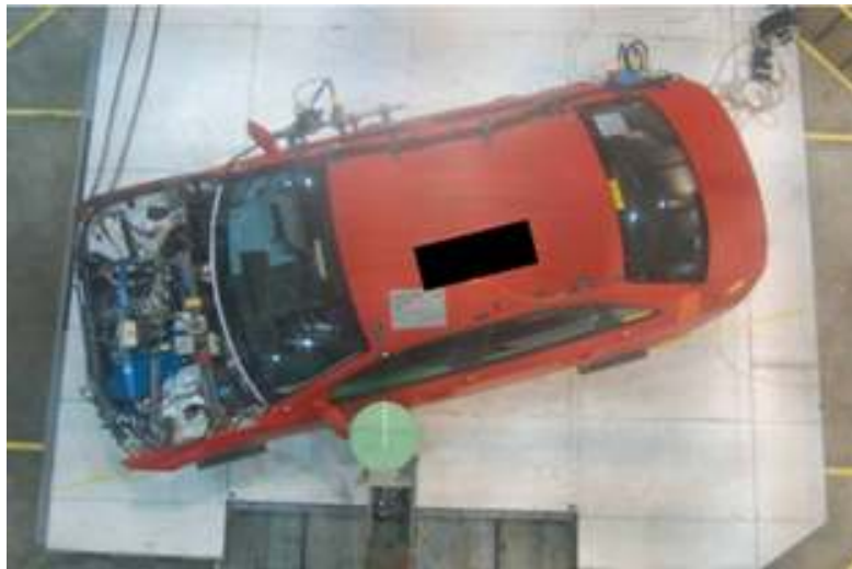
Figure 14: Top view oblique pole crash set-up
