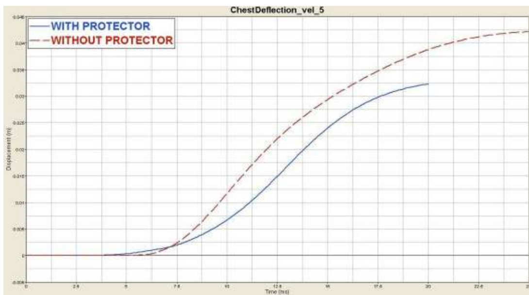
Fig. 12 – Chest deflection at 5 m/s cylindrical impactor
