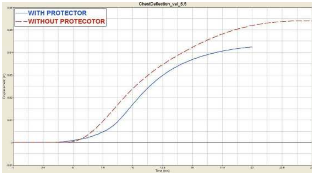
Fig. 13 – Chest deflection at 6,5 m/s cylindrical impactor
